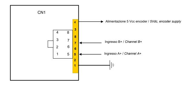
Gli encoder utilizzabili sono: onda quadra 0-5 Vcc push pull, o open collector PNP. *Encoders that can be used are: 0-5Vdc push pull, open collector PNP.*
